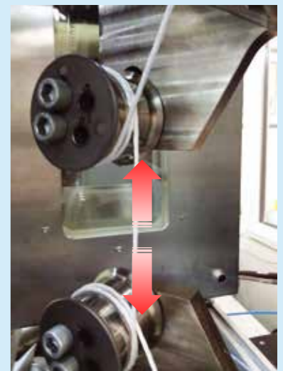
Setup for rope yarn Abrasion Test: Steel roller grips in cyclic motion
