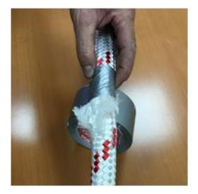
• Wrap the damaged length with the NikaPolyester-web cloth, folding the sides back in order to tightly fit the rope's circumference.
