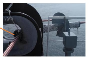
• NIKA-Protector is usually installed before the eye-splice construction of a new braided rope but can be also easily fit into an already used rope.
