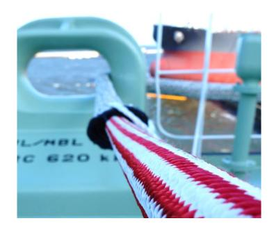
Make sure that the braided length of the NIKA-Protector is in contact with the chock. Otherwise there is risk of damaging the ending plasticized parts of the NIKA-Protector.
