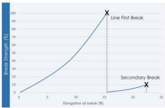
The higher elongation of the RSB member results in a two-step rope partition and reduces the extreme snap-back effect.
