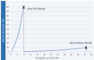
The higher elongation of the RSB member results in a two-step rope partition and reduces the extreme snap-back effect.
