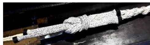
Cow Hitch connection of UHMWPE NIKA-SIRI@ S-12 with NIKA Nylon tail
