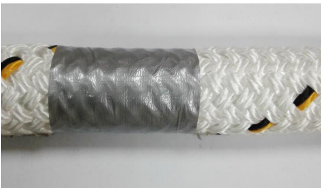
Temporary repair with adhesive tape
