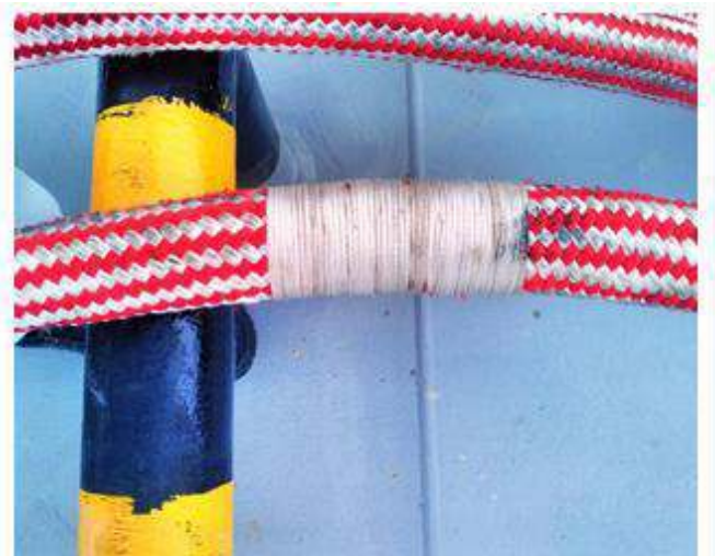
Small repair by whipping
